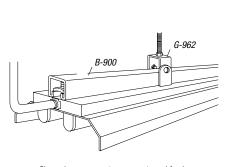
Channel raceway system supports and feeds fluorescent lighting fixtures.
