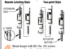
Keeper can be adjusted 3.2 (.13) from center both vertically and horizontally for proper alignment with latch.
