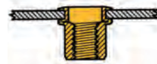
The reverse trigger is depressed and the tool unthreads from the installed fastener.
